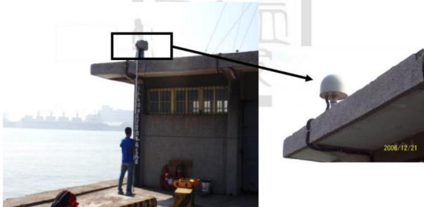
Figure 4-3 Configuration of GNSS station in Kaohsiung harbor
