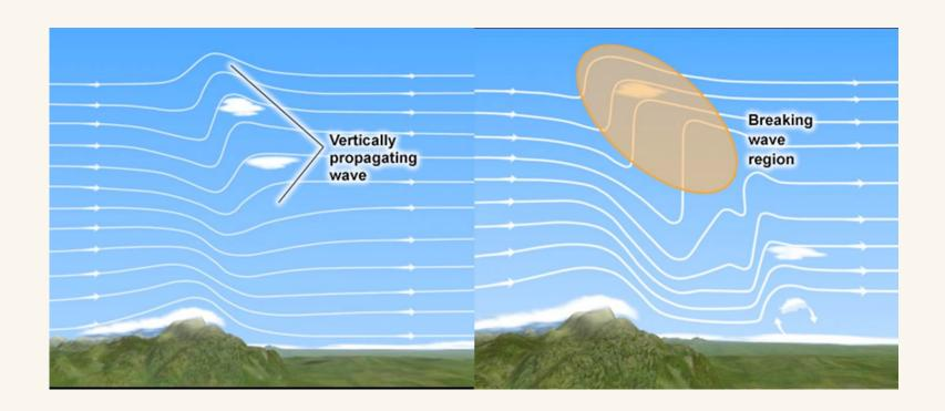
Vertical propagating waves excited by the topography may break under certain atmospheric conditions and hence it needs to be represented in the model, especially when grid sizes are larger than 5 km. Low level flow blocking are also parameterized.
